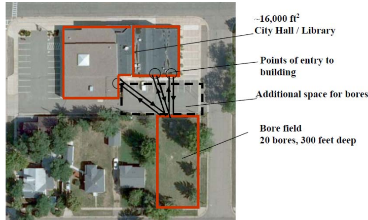
Figure 5. City Hall/Library Geothermal Bore Field Layout
